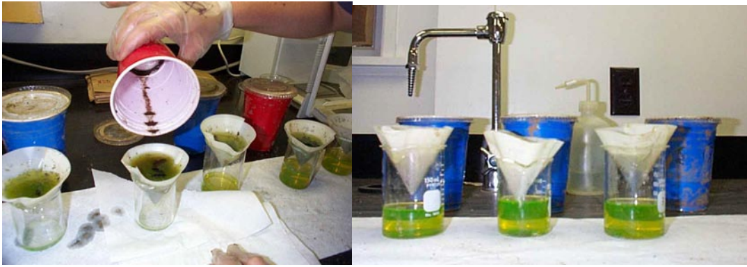
Figure 3. (A) Pit fall trap cups were emptied into labeled filter paper funnels that were placed into glass beakers. (B) Antifreeze drains through the filter paper funnels into the glass beakers; filtered antifreeze was then placed back in pit fall traps in the field.
